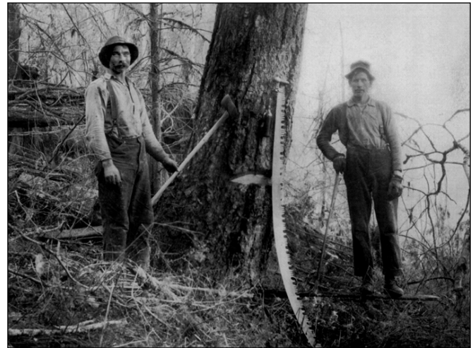
Joel (standing on springboard at right) and Charles "Carl" Brandt on left, ca. 1910-1917. The two-man bucksaw leaning against the tree was called a "misery whip."
